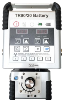
GIERTH TR90/20 Battery Battery powered X-ray unit
